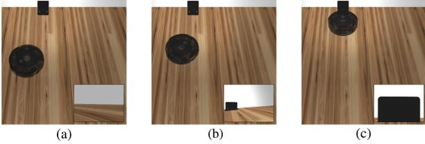
Figure 3: A sample episode from the docking simulator using a fully trained policy. The perspective of the front-facing camera is shown in the bottom-right of each image. (a) The robot is initialized in a random position. (b) The robot turns to face the dock. (c) The robot successfully docks.
