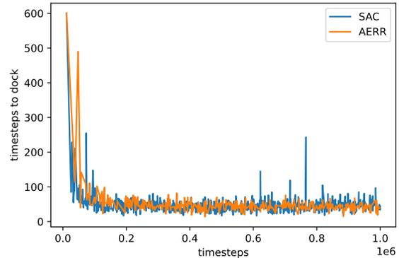
Figure 6: The performance of the AERR and baseline SAC algorithm on the simulated environment, in terms of the time taken to successfully dock. While we found these results to be stable over multiple runs, we caution that the preliminary results presented here represent a single run and that the level of uncertainty has not been quantified.
