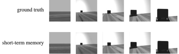
Figure 1: Reconstruction of the short-term memory of a simulated robot vacuum with a front-facing camera docking using the proposed method. The history of observations is recursively compressed into a vector which is given as input to a reinforcement learning policy. This vector can be recursively decoded to reconstruct the original camera images.
