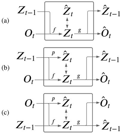
Figure 2: Three types of AERR units. The dotted line indicates the use of the KL divergence. (a) shows the system with an unconditioned prior. (b) shows the system with the forward dynamics prior. (c) shows the system with the associated memory prior.
