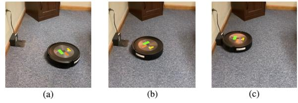
Figure 4: A sample episode from the real-world docking environment using a fully trained policy, similar to the simulated episode in Figure 3. We see the same basic steps: (a) The robot is initialized in a random position. (b) The robot turns to face the dock. (c) The robot successfully docks.
